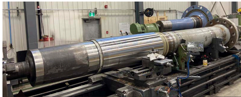
TURBINE SHAFT Refurbished (Ø45" x 21 feet long / 33 000LBS)
