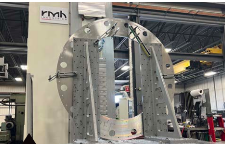
NEW STAINLESS STEEL FACING PLATE Ø8'
