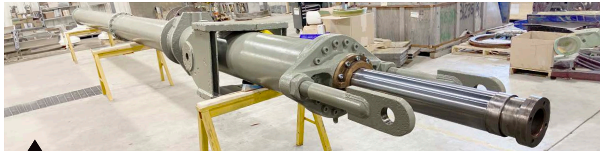
WATER INTAKE GATE CYLINDER Rehabilitation (78' extended)
