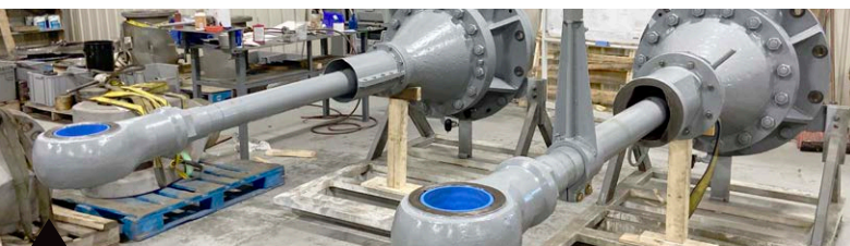
Servomotors refurbished with THORPLAS-BLUE bushings
