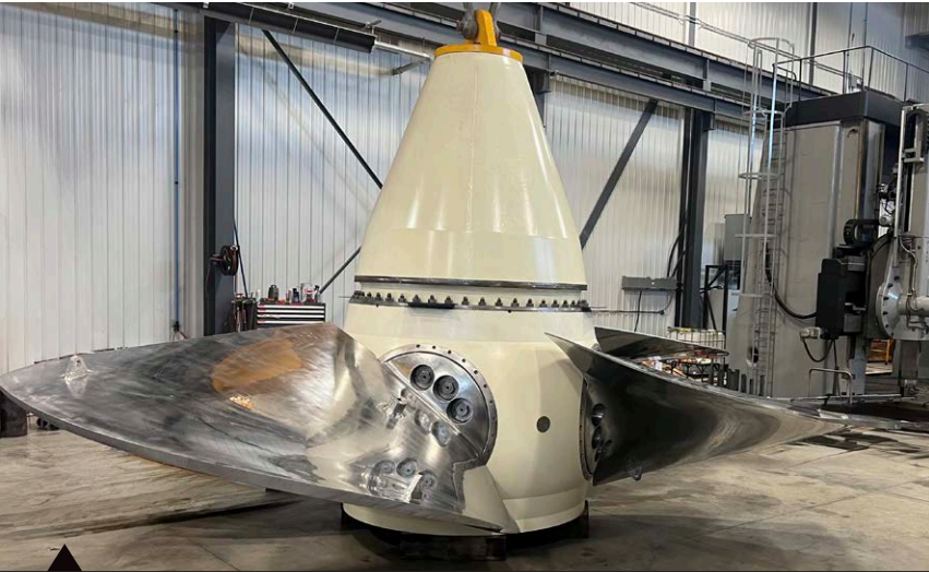
KAPLAN RUNNER Refurbished and tested (55 tons)
