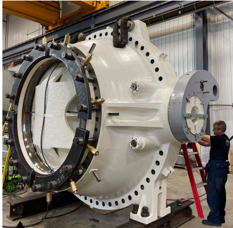
MAIN INLET VALVE Refurbished and tested (65 tons)
